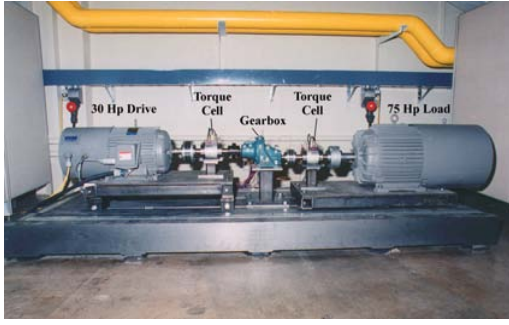
Fig. 5. Mechanical diagnostic test bed.
